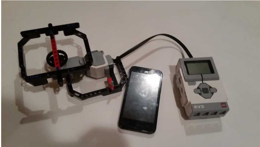
Figure 2. The test bed used to collect sensor data while the phone is rotated. A LEGO Mindstorms EV3 system is used to drive the rotation.
